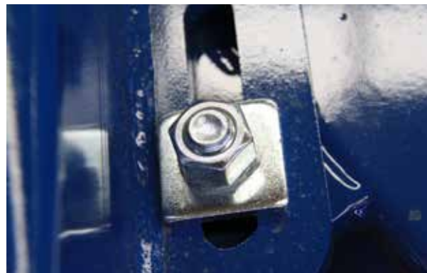
Remove the bolt and pin from each gang
