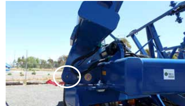
figure g7 Wing Pivot 2 points per side as required
