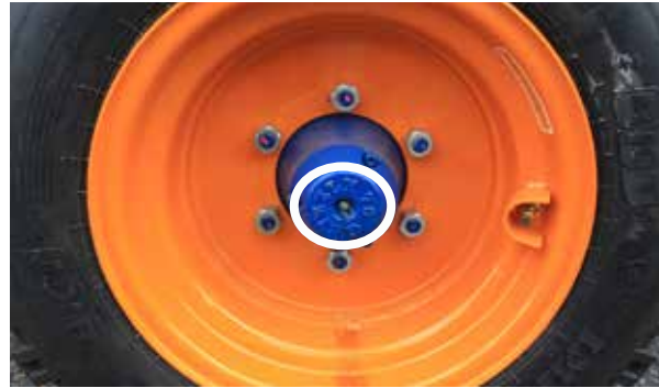
figure g3 Wheel hubs 4 point weekly
