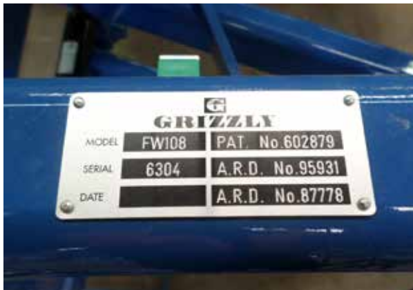
Above: The serial number plate is located at the front of the main frame.
