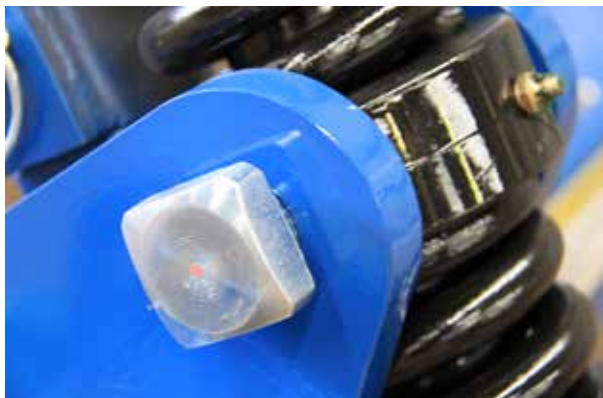
Loctite bolts use high strength loctite
