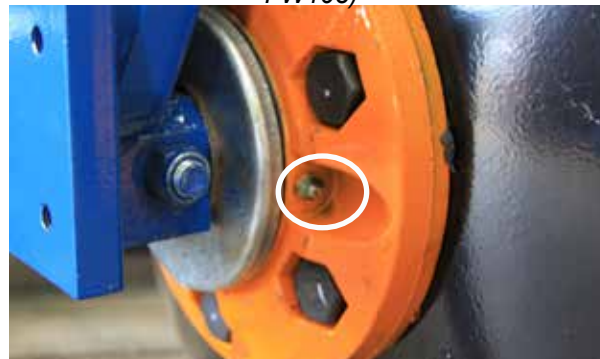
figure g5 Disc gang bearings daily 1 point per hub
