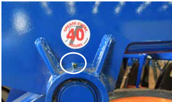
figure g2 Wheel pivots 2 points per gang as required
