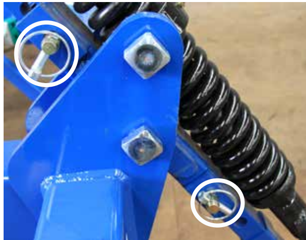
Lock Up Bar in Transport Position
