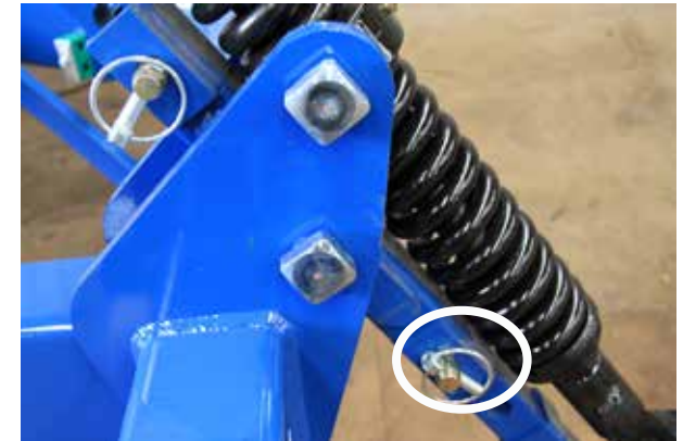
Pitch lock pin, for transport only. Remove when working
