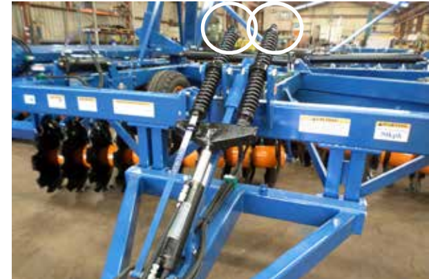
Correctly adjusted the top springs have 30mm of thread extending through the lock nut.
