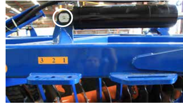
figure g6 Wheel lift cylinders 2 points each weekly
