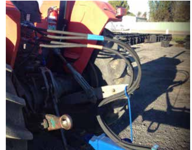
Hoses reversed through holder, out of harms way
