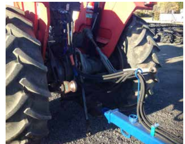
Hoses hanging too close to draw bar pin
