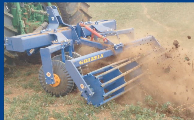
WTR06 in operation at 12km/h
