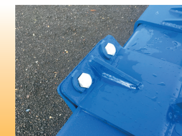
Captive bolts make maintenance and adjustments easy.
